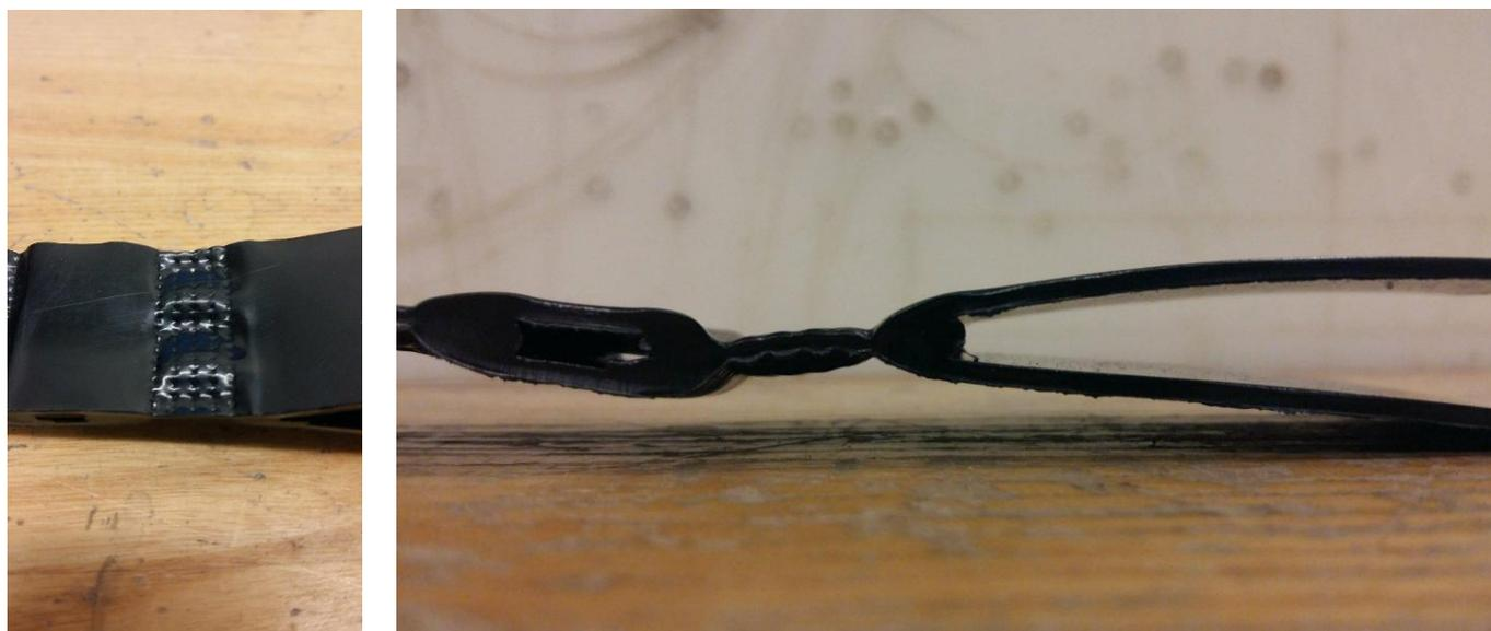
Figure 2. Cross section of a weld 1 shear specimen. Note rippling on weld track as a qualitative indication of overheating.
