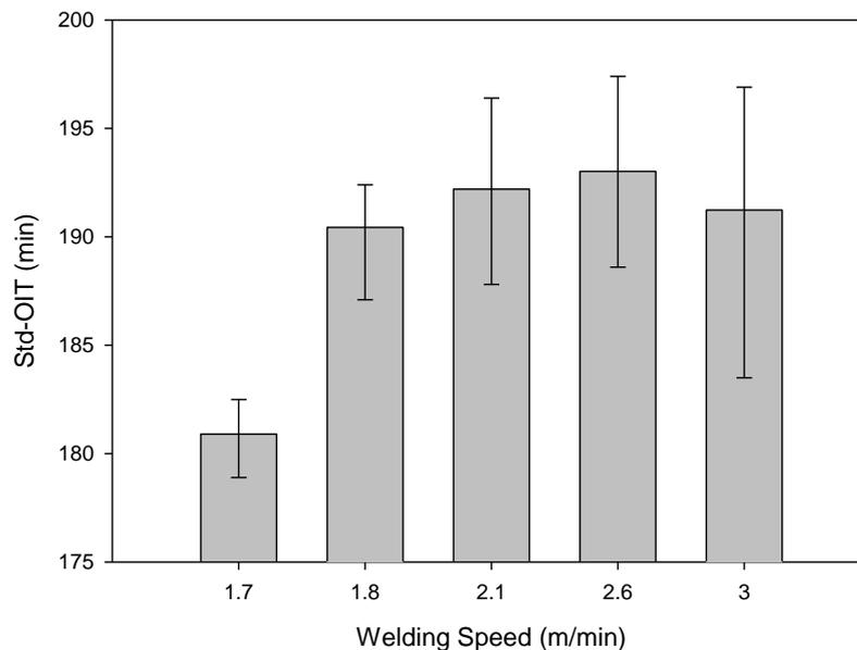
Figure 4. Variation in HAZ Std-OIT categorized by welding speed. Error bars represent the range of values for a given speed.
