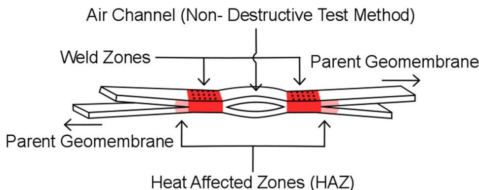
Figure 1. Cross section of typical HDPE dual track fusion weld.
