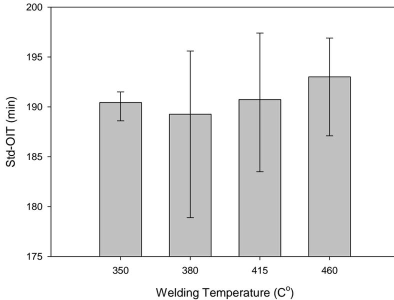
Figure 3. Variation in HAZ Std-OIT categorized by welding temperature. Error bars represent the range of values for a given temperature.
