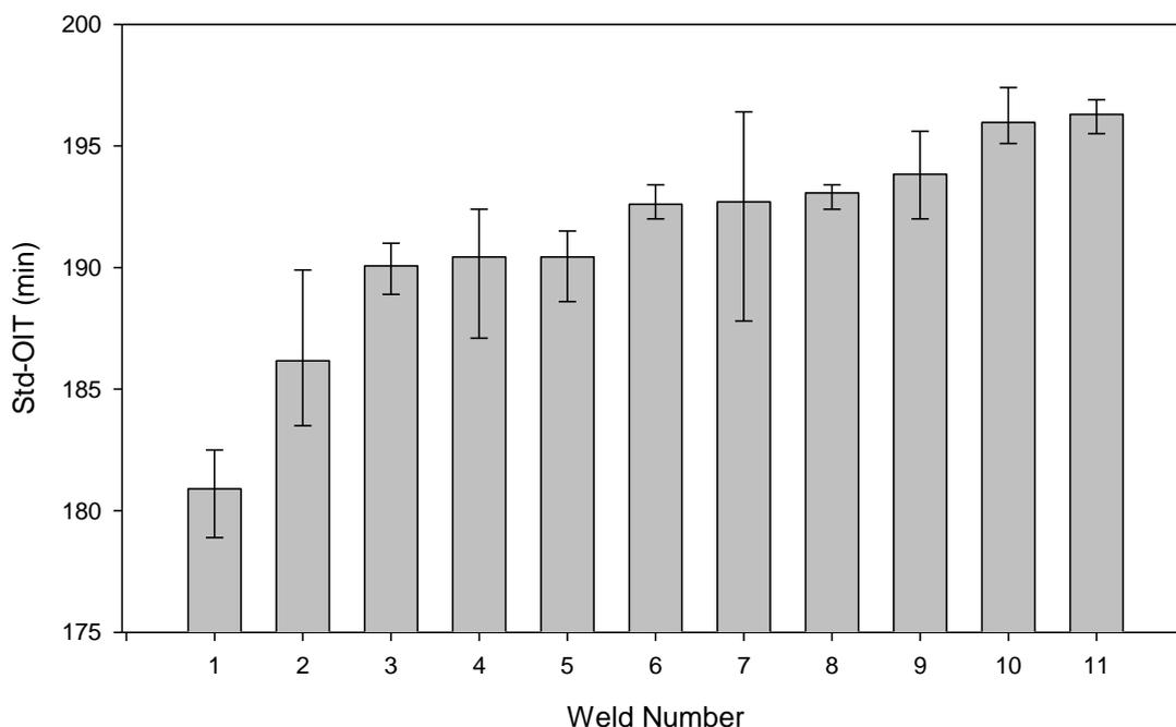
Figure 4. Variation in HAZ Std-OIT categorized by welding speed. Error bars represent the range of values for a given speed.
