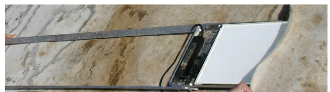
Fig. 18. Thin (300 × 300 × 8 mm) LED light panel attached to tray being inserted below a panel at an overlap using push-pull rods.
