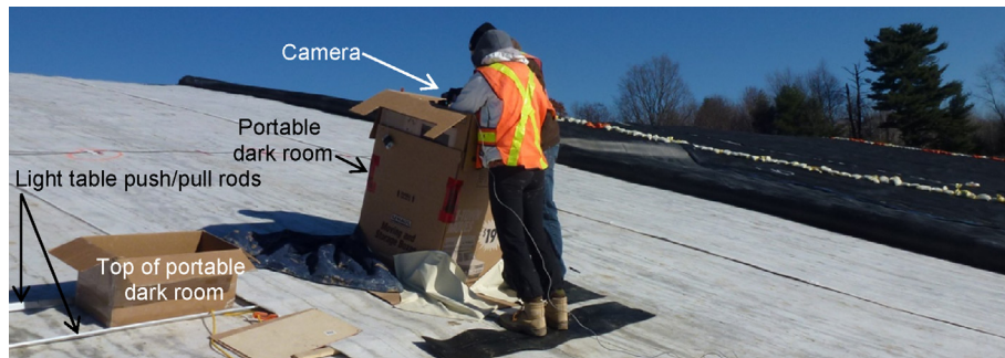
Fig. 19. Camera being set-up in portable dark-room after insertion of light table to the target location. Once camera is set up, the top of the dark room was placed and the camera triggered remotely.
