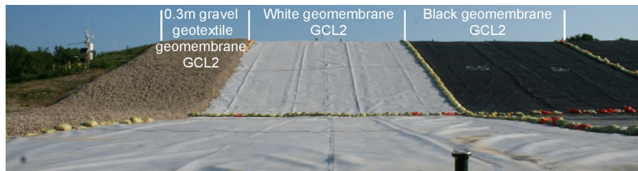
Fig. 16. Western three sections of QUELTS II viewed looking north. From west to east (left to right): [1] GCL2 covered by black geomembrane, geotextile protection layer, and 0.3 m gravel, [2] GCL2 covered by a white geomembrane, and [3] GCL2 covered by a black geomembrane.
