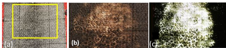
Fig. 13. GCL3 with black woven-up and irrecoverable erosion 'EE': (a) photographed with a halogen backlight in normal daylight, (b) close-up of 200 mm wide area inside box shown in Figure 13a photographed with halogen backlight in normal daylight, and (c) close-up of the same area as Figure 13b with the same halogen backlight but photographed in a dark room. The black areas in Figure 13c are where there is still a significant thickness of bentonite. Modified from Ashe et al. (2015).
