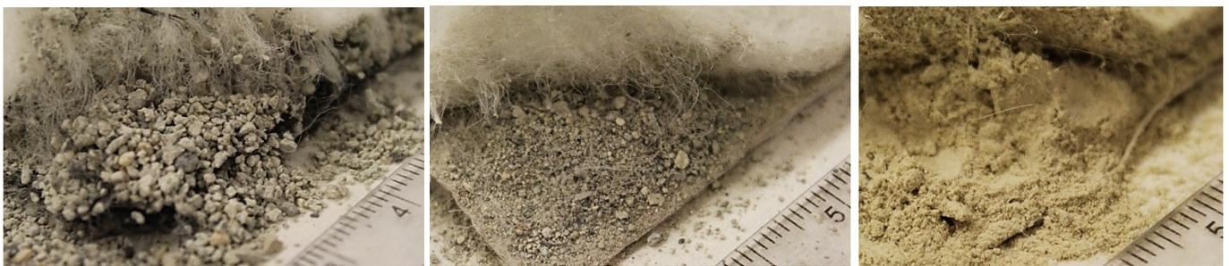
Figure 1. Deconstructed GCLs with coarse granular, fine granular, and powdered bentonite. Scale in cm.
