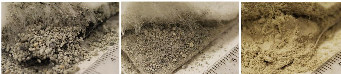
Figure 1. Deconstructed GCLs with coarse granular, fine granular, and powdered bentonite. Scale in cm.
