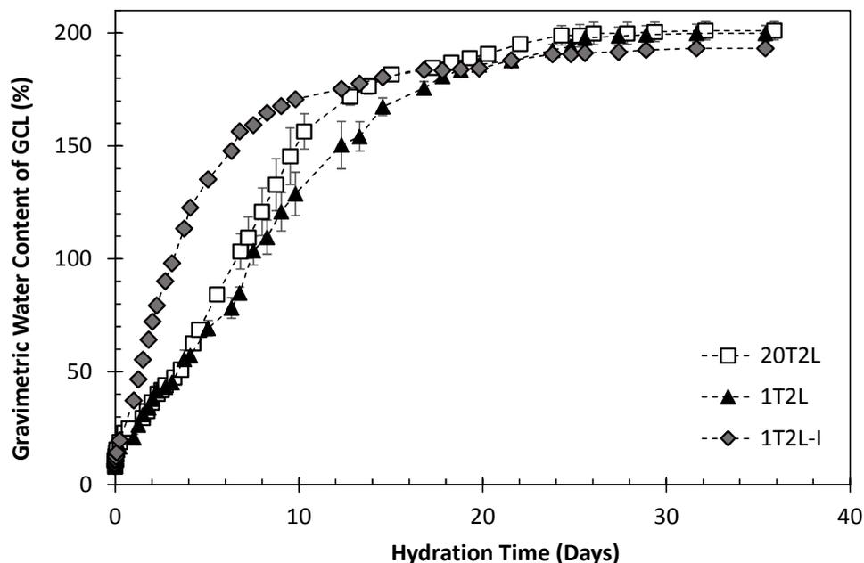
Figure 1 - Gravimetric water content versus hydration time of GCL conditioned at +20°C (20T2L), +1.5° (1T2L) and with ice formed in the carrier (1T2L-I).
