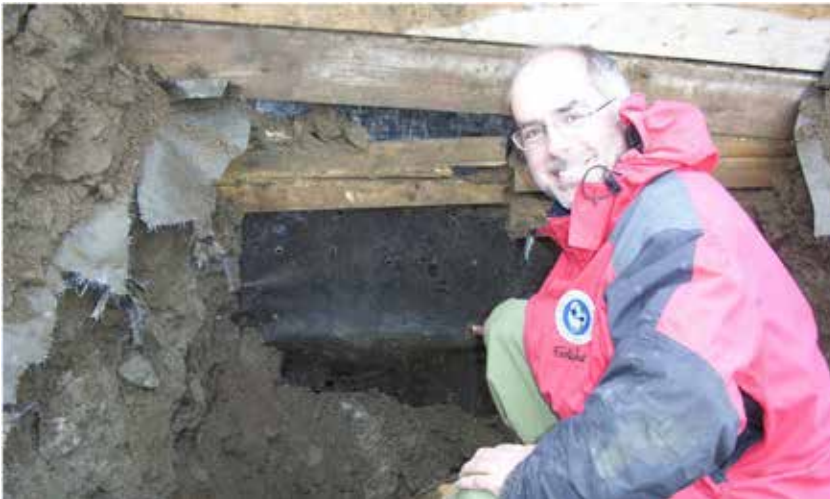
Bathurst excavating buried geomembrane test samples at the location of a subsurface oil spill at a DEW line site in the Canadian Arctic.
