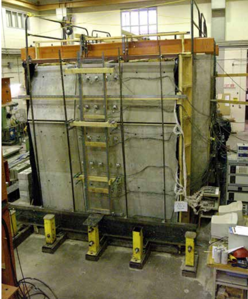
An incremental panel wall taken to failure under surcharge in the RMC full-scale retaining wall test facility.
