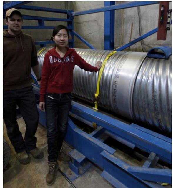
Yu Wang with Civil Technologist Graeme Boyd using the new pipe joint testing frame on corrugated steel pipe.
