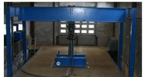
Culvert testing for tandem axle loads
