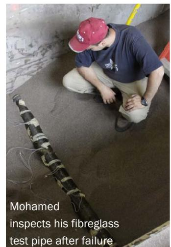
Mohamed inspects his fibreglass test pipe after failure
