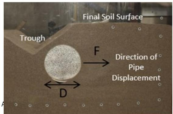
View of moving pipeline through the window part-way through a lateral pulling experiment showing the pipe, and changes in the geometry of the ground surface.
