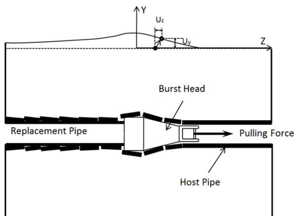
*Schematic of the pipe bursting process*
