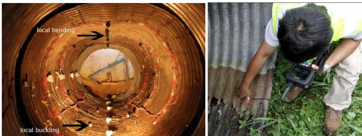
*Failure mode for culvert tested to its strength limit Van measuring thickness in the field.*
