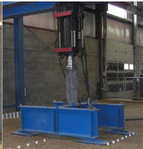
Use of the GeoEngineering Laboratory to conduct full scale testing of a large span metal culvert under both real and simulated truck loading.
