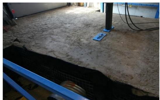
*Surface load test on a 0.9 m diameter corrugated steel pipe*
