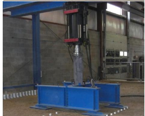
*Surface load simulating tandem axle
