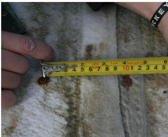
Figure 3. Photograph of machine screws used to record movement of GCL overlap. The initial separation between the screws at this location of a GCL2 overlap was 10 cm. This photograph was taken 2.2 years after construction and shows no discernable increase in separation between the two screws since construction.
