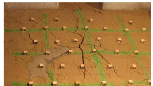
Ground surface after hydrofracturing in the large scale laboratory tests
