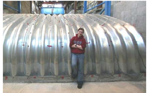
Andrea and her test culvert prior to backfilling in 2008.
