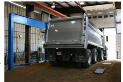
Culvert testing under a heavily loaded dump truck in 2008.
